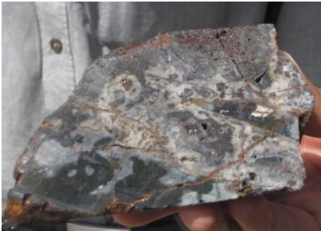
Figure 5 AD016 – Core sample (31% Sn)
